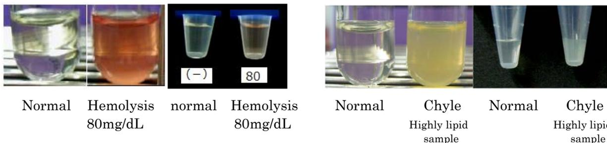
If presence of interfering substance is suspected, examine by dilution test at more than 2 points. Dilution of a sample should be made in a test tube using buffer solution prior to adding them to wells.
